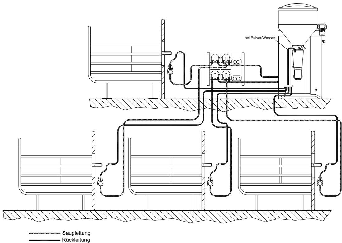
The extension of 4 feeding stations SynchroFeed includes a flow adapter with four connections used for the return lines.
