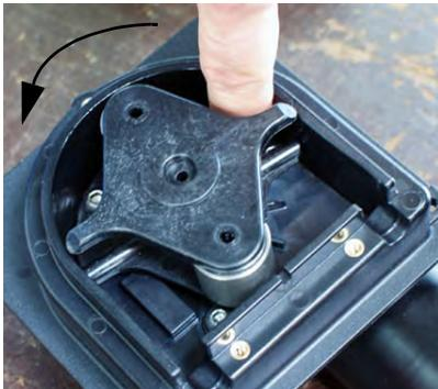
6. Clamp the supplied pump hose between the housing and the roller of the rotor. Position the pump hose by turning the rotor counter-clockwise so that it is centered on the roller.
