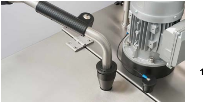
1 Cleaning head in tank lid
