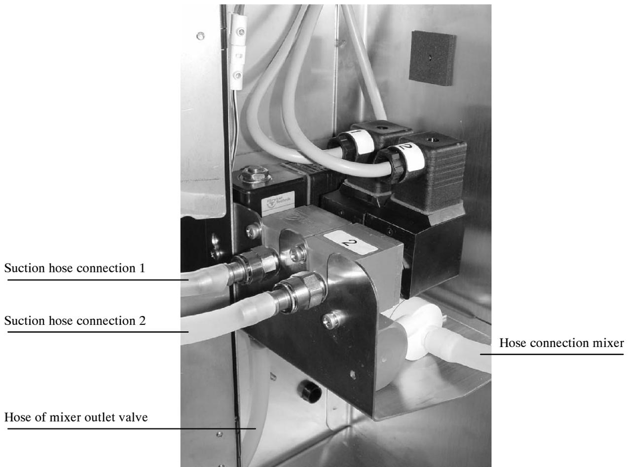
***Take care that suction hose connection 1 runs to feeding station 1 (identification 1) and suction hose connection 2 runs to feeding station 2 (identification 2). In case you should not observe this order, a calf trying to get its milk portion at feeding station 1 will get no milk because the milk portion will be distributed at feeding station 2 instead.***
