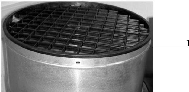
1 Hole on the top section of the powder hopper to screw in a self-cutting screw.
