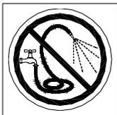
Wipe the automatic feeder only with a moist cloth. Never use a high-pressure cleaner or similar to clean the automatic feeder.
