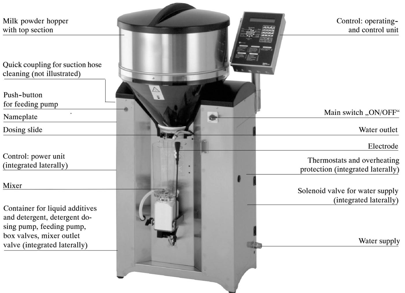
Dimensions of the automatic feeder: Height = approx. 1260 mm, width = approx. 720 mm, depth without additive dispenser = approx. 570 mm, depth with additive dispenser = approx. 660 mm.
