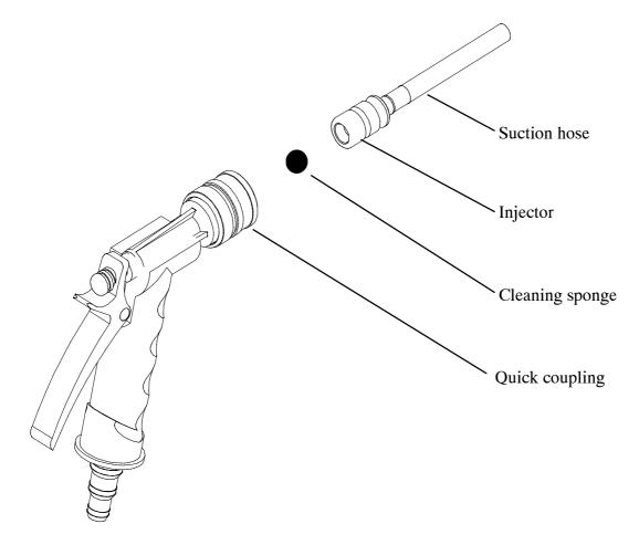
**Note:** The solenoid valves resp. the pressure sensors and the pump have to be cleaned solely with clear water. Never use the cleaning sponge because it may lead to clogging thus damaging the above-mentioned components!
