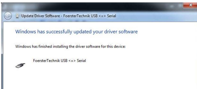
Now the **virtual COM-port-driver** must be installed.
