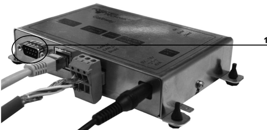
1 Serial RS232 interface (9-pole): Slot for null modem cable for gateway
