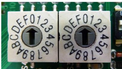
1. Set Pump 1 using hex switch S4. The arrow points to the set pump duration.
