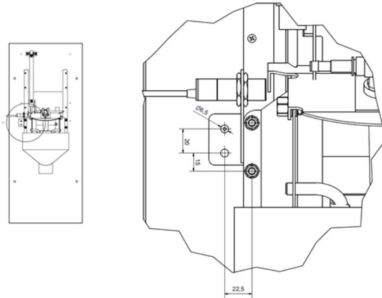
2. Attach the sensor holder to the teat slider's front plate.
