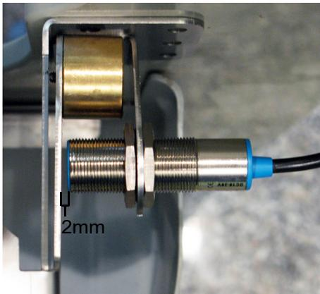
6. Run the sensor cable to the control unit. Attach a ferrite one meter after the sensor (see machine wiring diagrams) and fix it to a wall.
