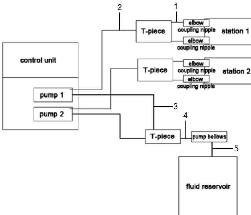
3. Install the cut to size hoses as sketched schematically in the figure.
