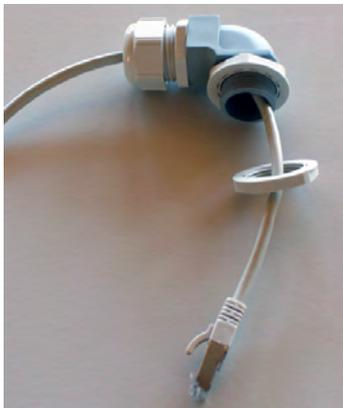
10. Guide the Ethernet cable from the outside in through the feedthrough of the new control box cover and push the angle piece into the cover.
